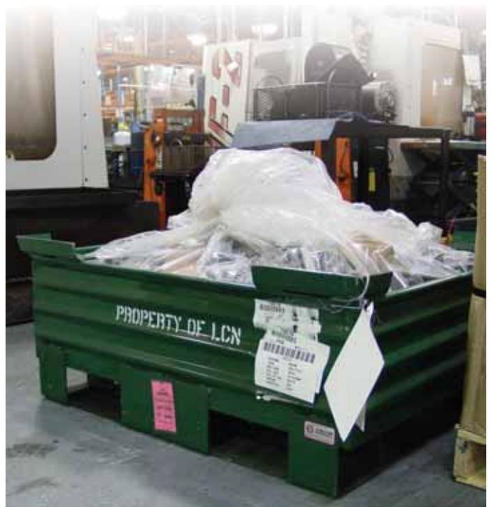
ers are formed from heavy 12 gauge steel, weigh approximately 260 lbs., and are built to handle a four thousand pound payload. Streater Dependable has provided LCN with these containers for the past 30 years.
