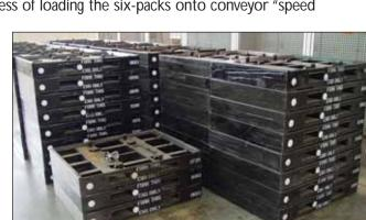
blocks were shipped to Streator so Dependable's engineers could design a pallet that was made-to-order, one strong enough to hold the engine blocks securely during shipping and one that would fit directly into International's staging area, thus eliminating any extra handling at the Melrose operation.
