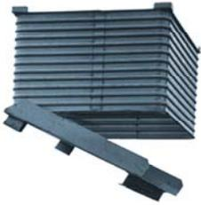
**Drop Bottom Box-** as it’s name implies the floor is hinged at the rear so when it is placed into a work stand it opens like a clam shell allowing the contents of the box to dump out.
